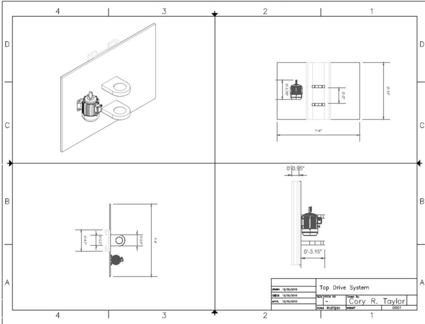
Figure 7: Top drive motor and carriage
