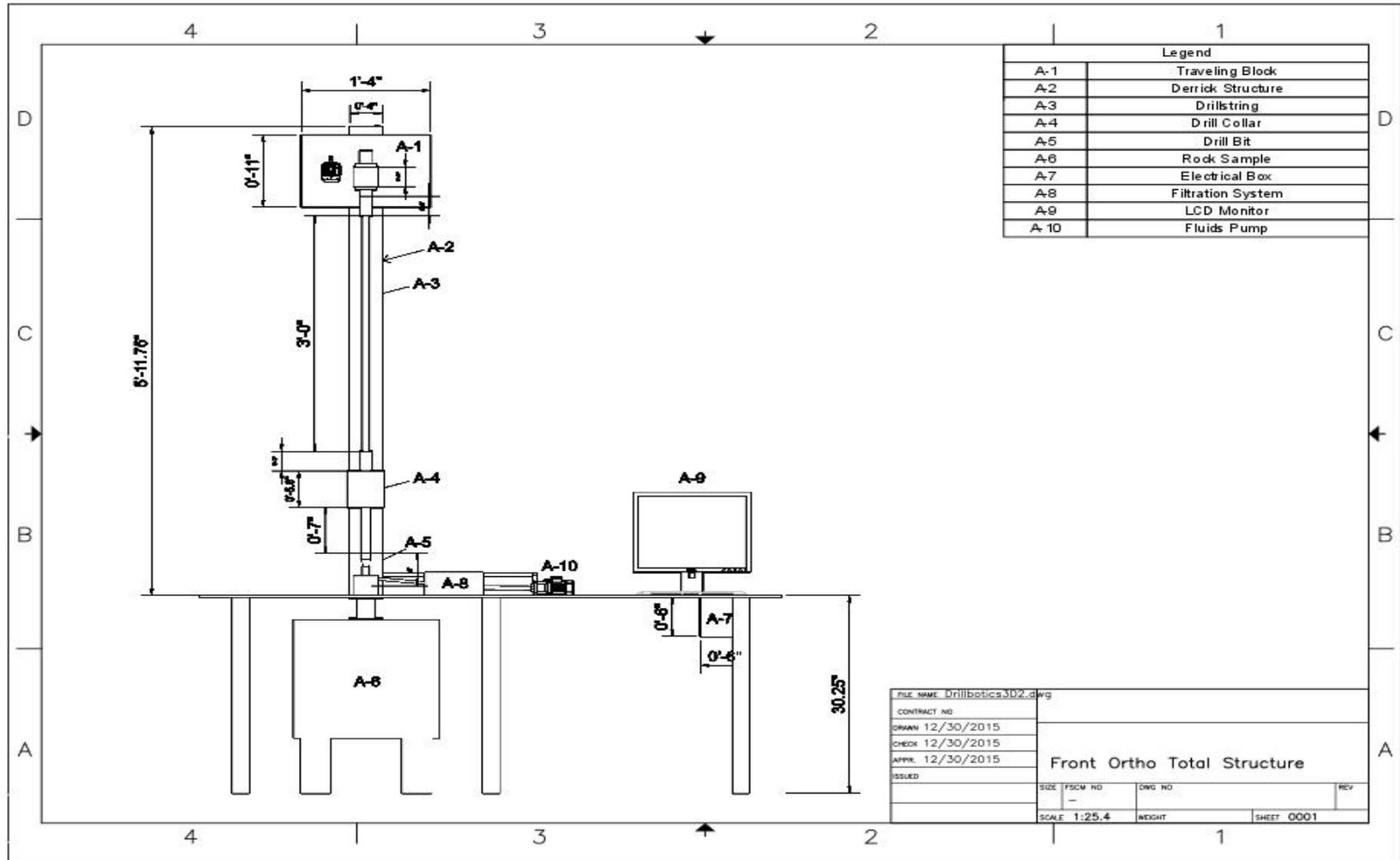
Figure 5: Front view of the proposed rig
