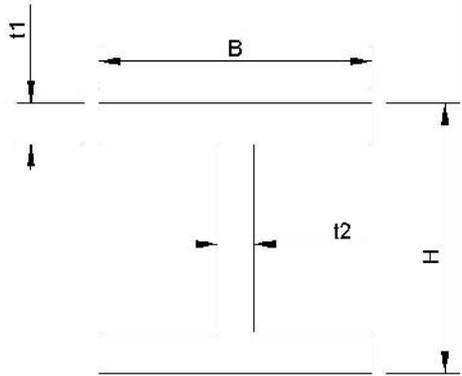
Figure 1: H-beam to be used as a guide for the moving block
