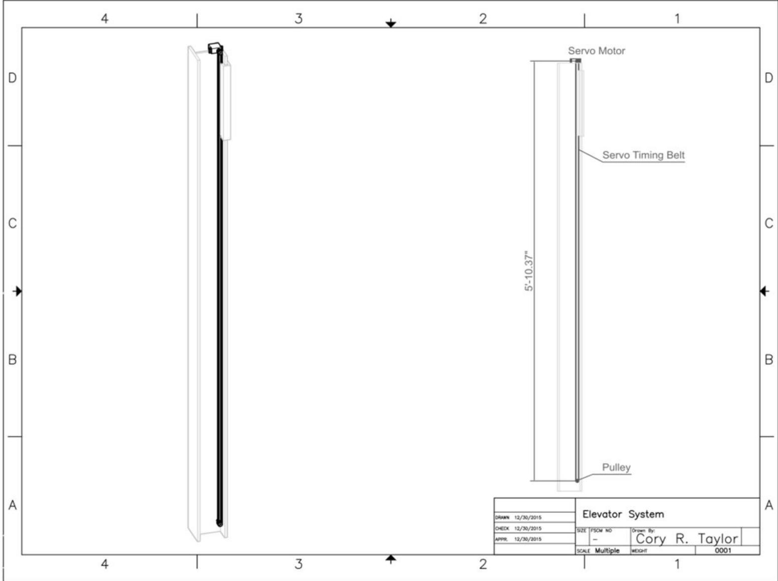
Figure 6: Proposed elevator system for linear displacement.
