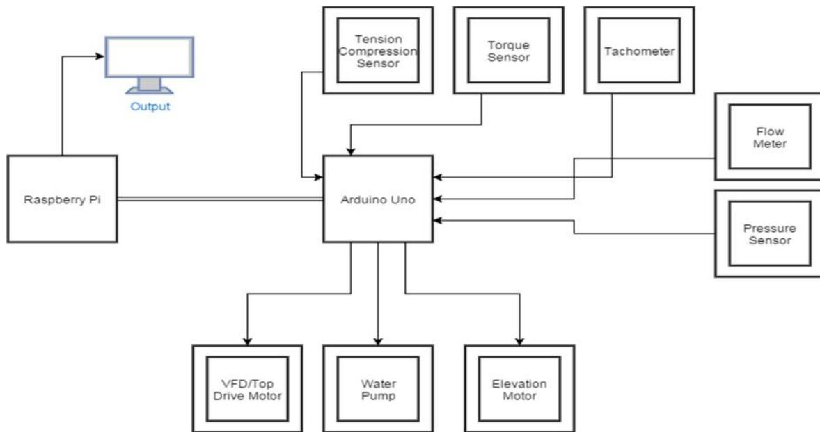
Figure 3: Block diagram showing proposed control system
