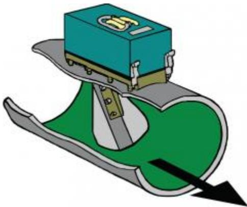
Figure 5: Flow-out Tracking Sensor
