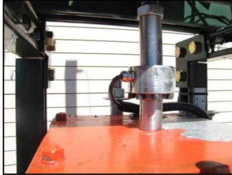
Figure 6: Load Cell
