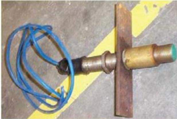
Figure 3: Flow-in Tracking Sensor
