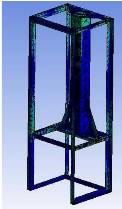
*Figure 4: Finite Element Analysis of the Drilling Rig Frame*
