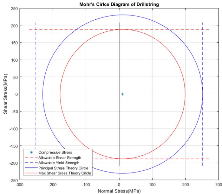
Figure 2: Mohr's Circle for Max Principal Stress and Max Shear
