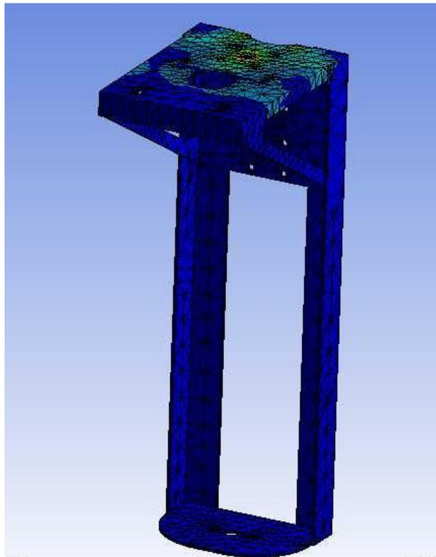
*Figure 7: Finite Element Stress Analysis of Drilling Platform*
