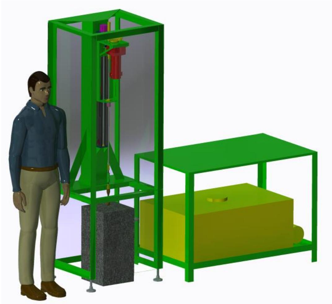
*Figure 3: 3D Render of Drilling Rig (Left) and Fluid Skid (Right)*
