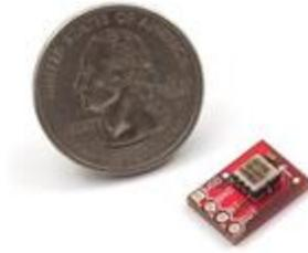
*Figure 15: Accelerometer and Breakout Board*
