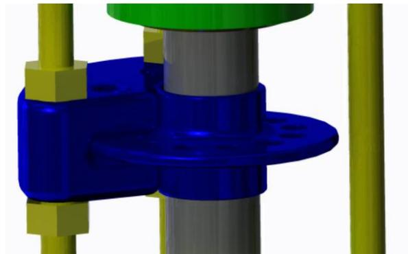
*Figure 14: 3D Printed Optical Encoder*
