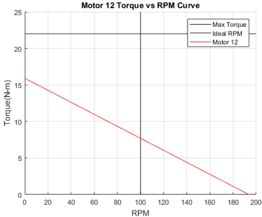
Figure 10: Drive Motor Torque-RPM Curve
