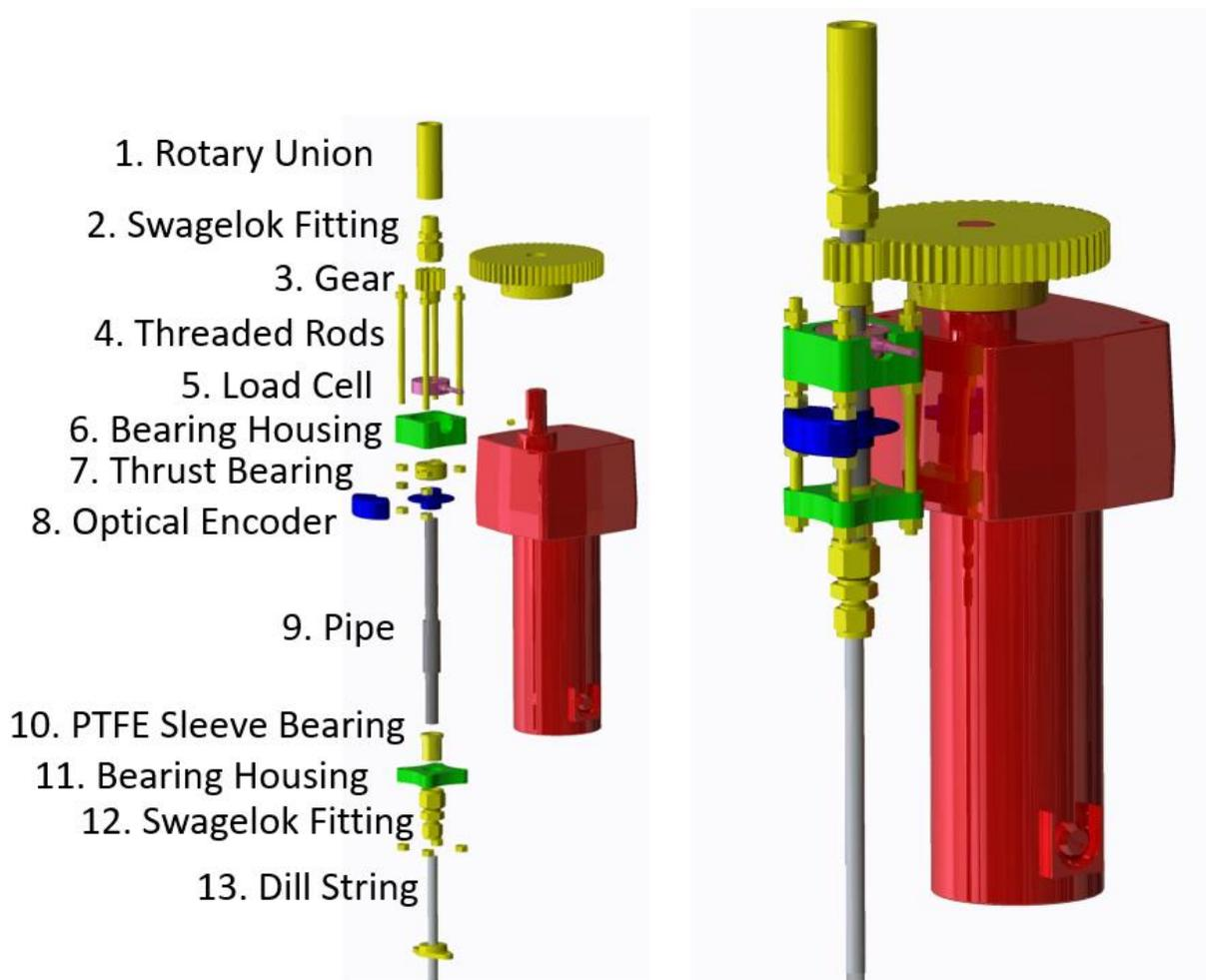
Figure 8: Exploded Swivel System
