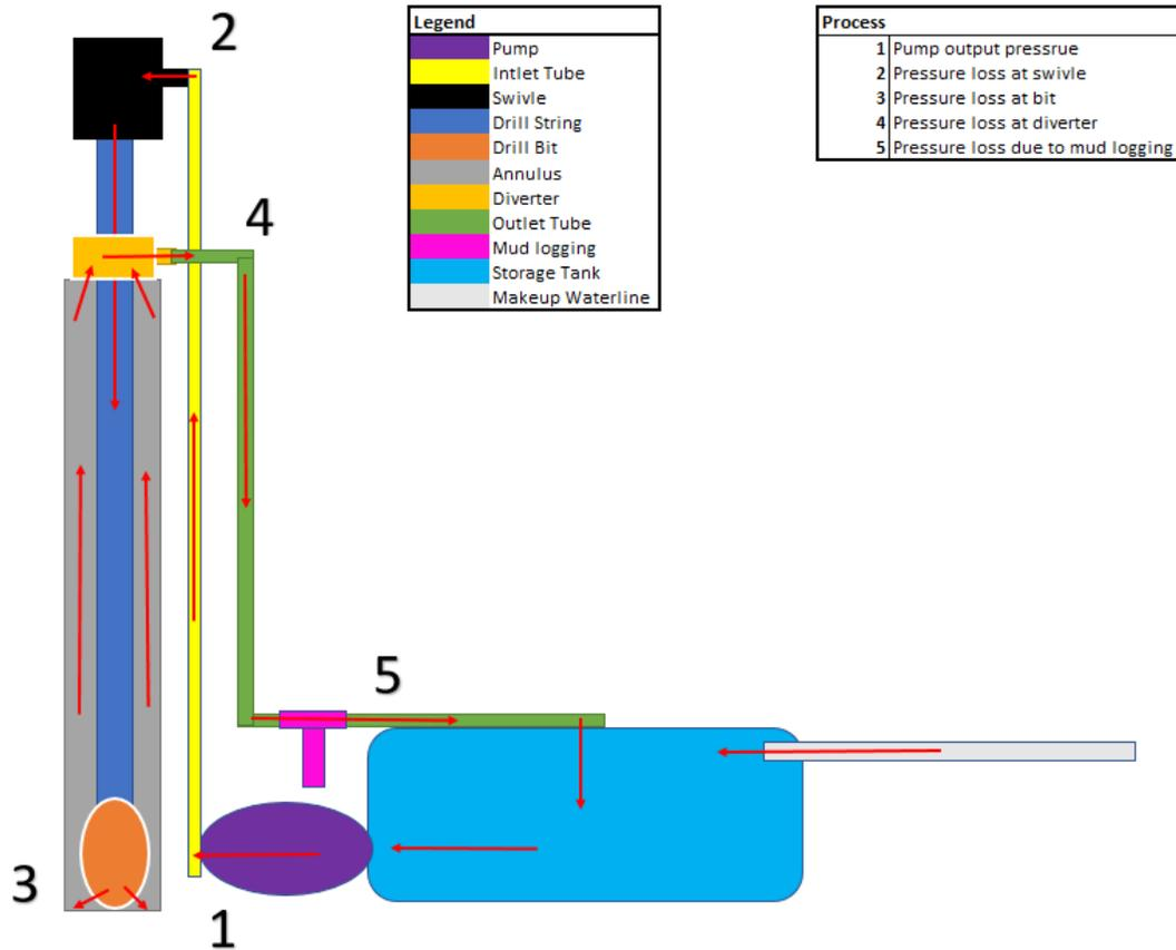
*Figure 12: Schematic Representation of the Fluid System with Nomenclature*
