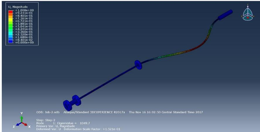
Figure 1: Finite Element Buckling Analysis of Drill String System.
