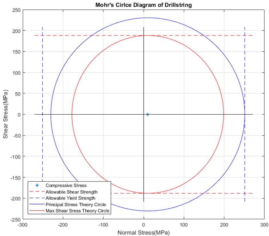
Figure 7: Drillstring' Mohr's circle for max principal stress and max shear.
