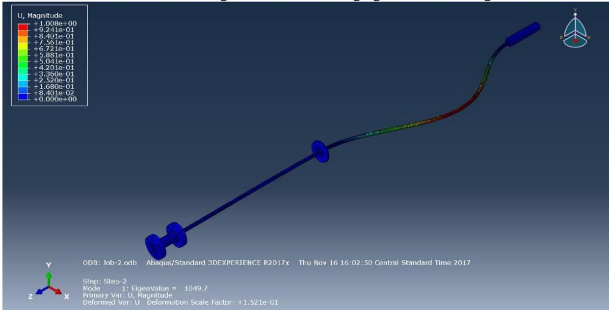
Figure 6: Finite element buckling analysis of drill string system.
