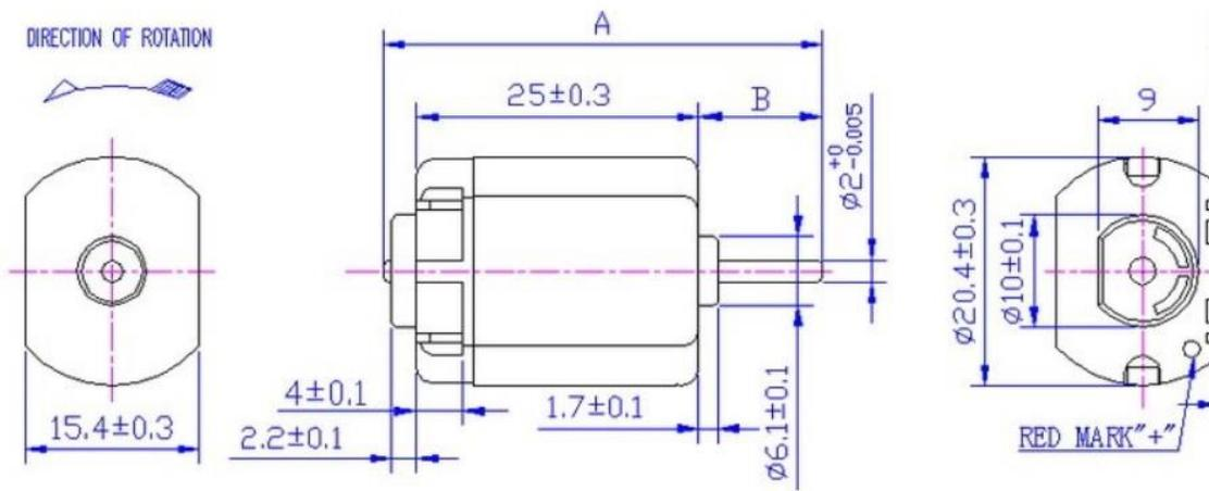
Figure 4: Dimensions of an example car mirror adjusting motor.
