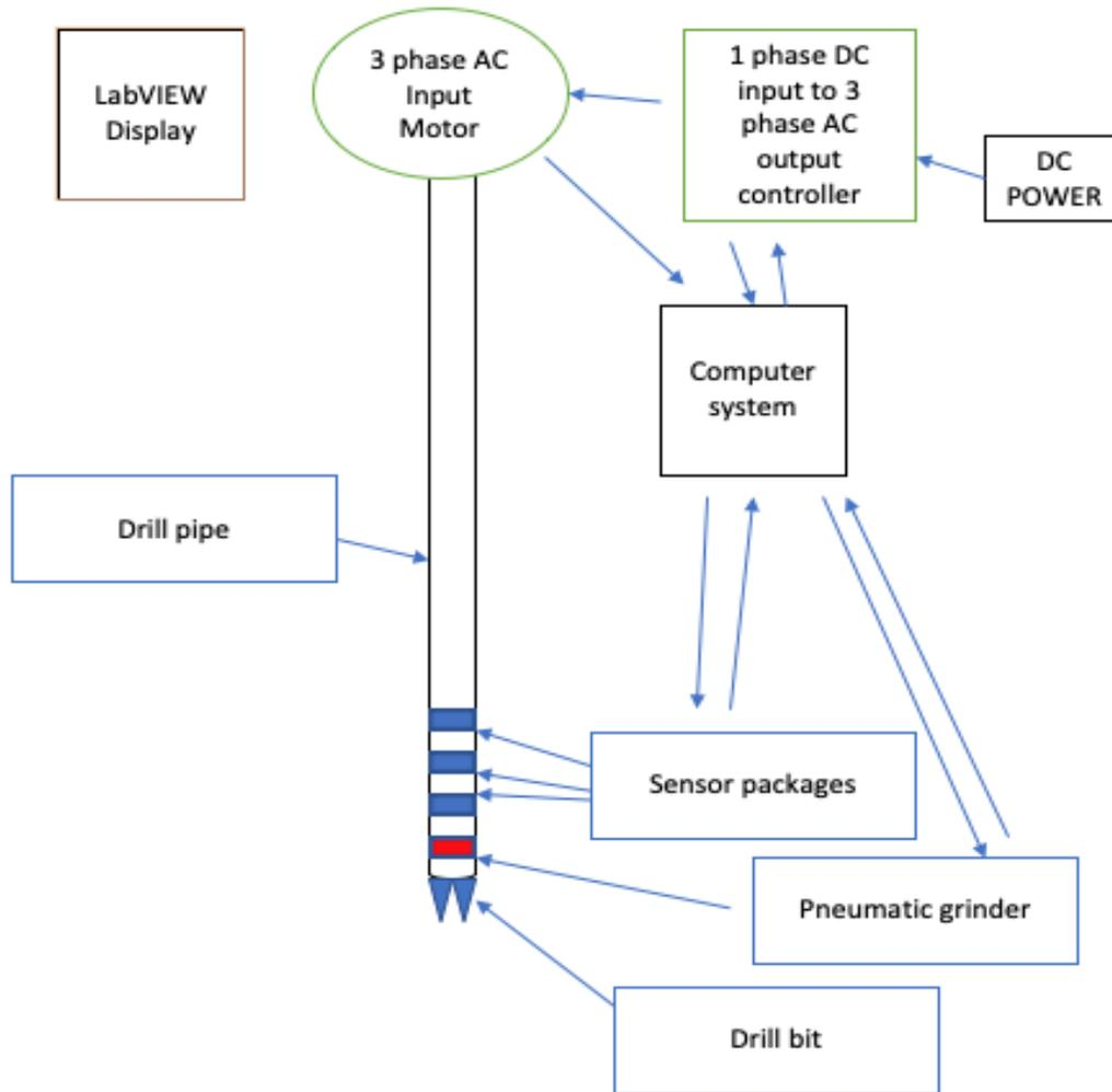
Figure 8: Schematic representing control system
