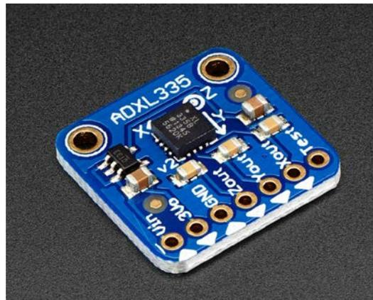
*Fig. 17: Accelerometer Measuring Vibration*
