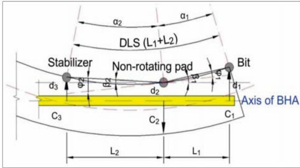
Fig. 5: DLS by push-the-bit mechanism
