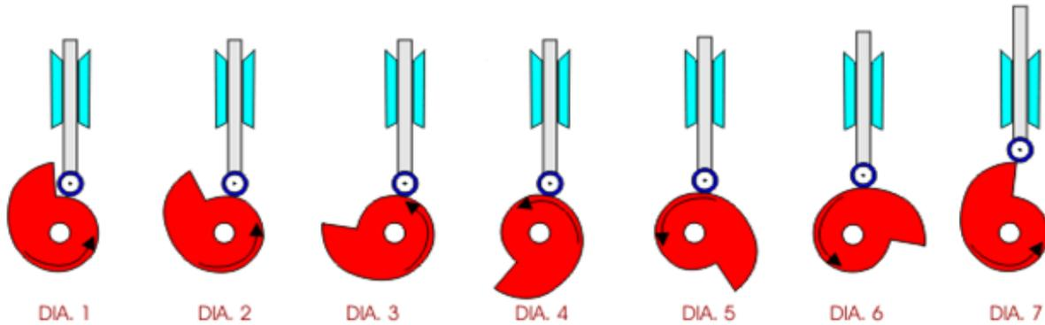
Fig. 3: working of Snail CAM
