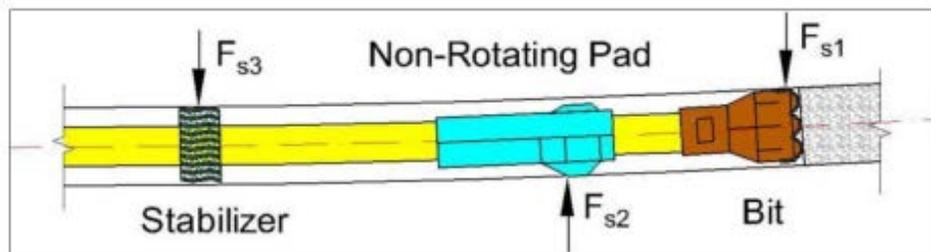
Fig. 4: Free body diagram of Push-the-bit setting
