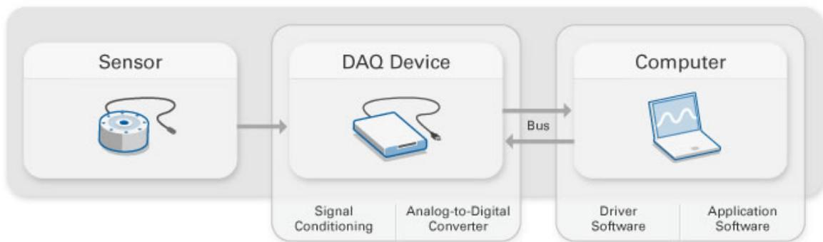
*Fig. 20: Data Acquisition System*
