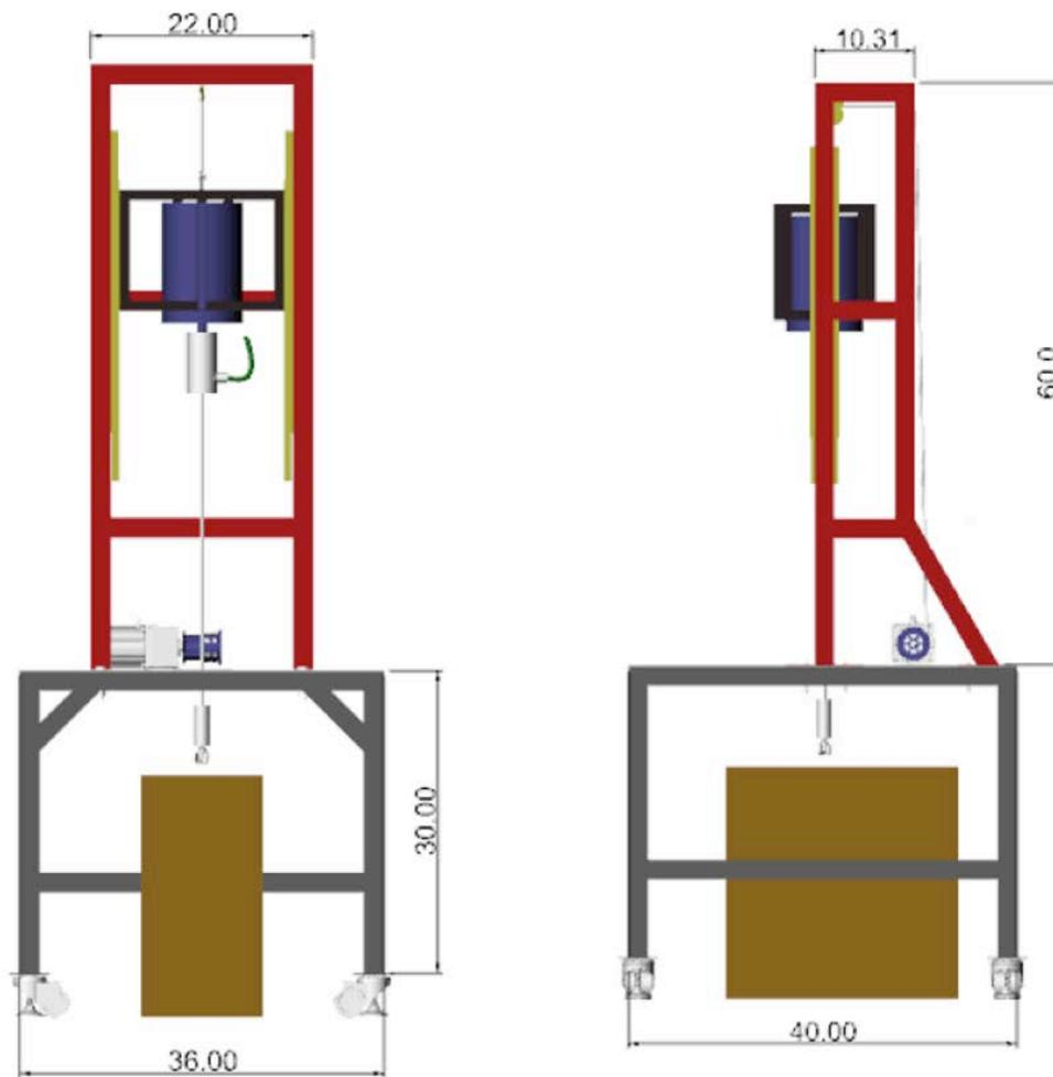
*Fig. 1: Shows main components and dimensions of the rig design*
