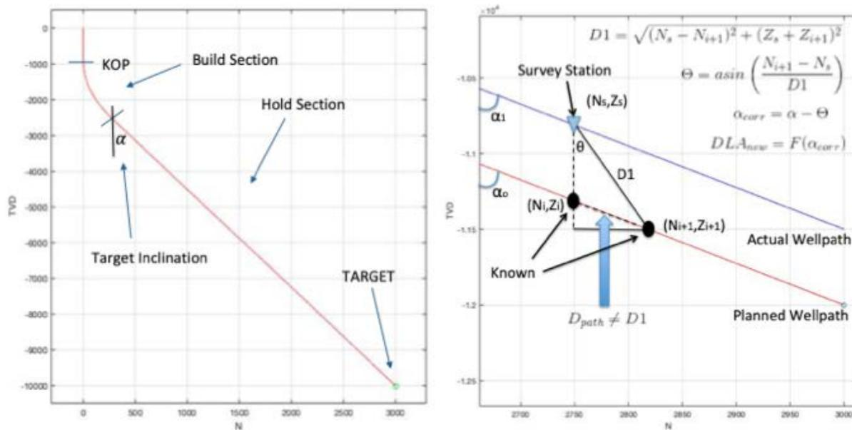
Fig. 23: (a) Example output of wellpath program (b) Theory behind wellpath correction
