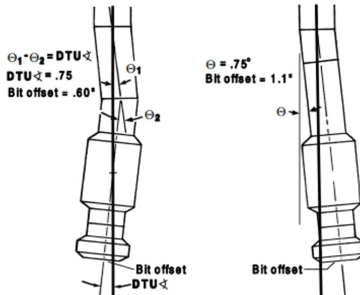
Figure 8: DTU & BIT offset
