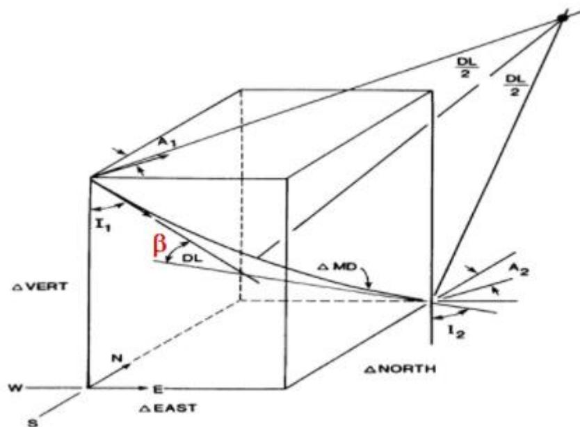
Figure 4: Minimum curvature method
