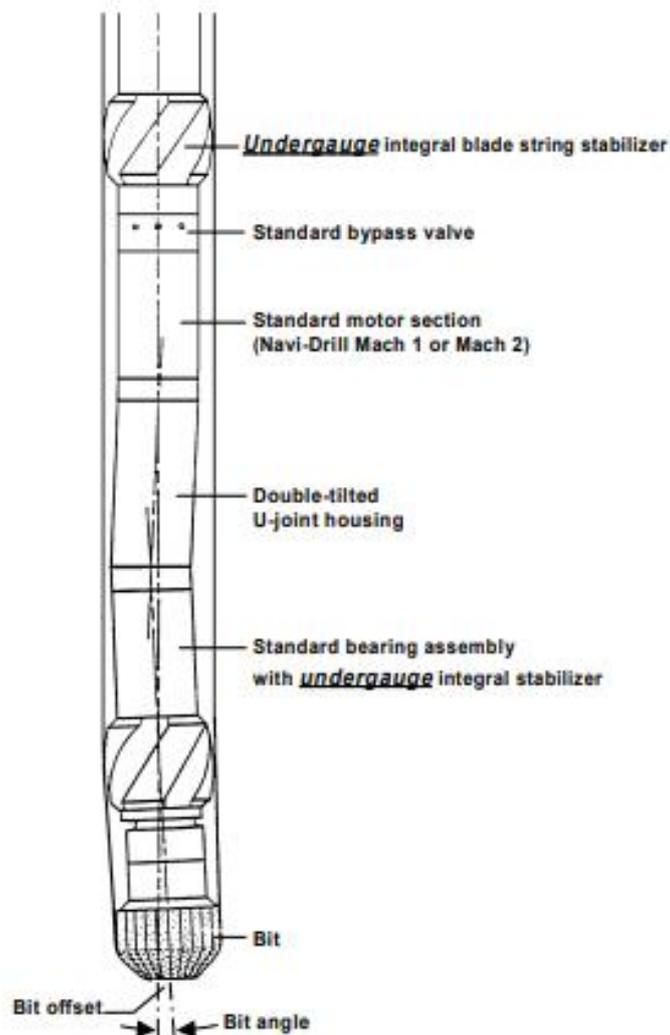
Figure7: DTU configuration
