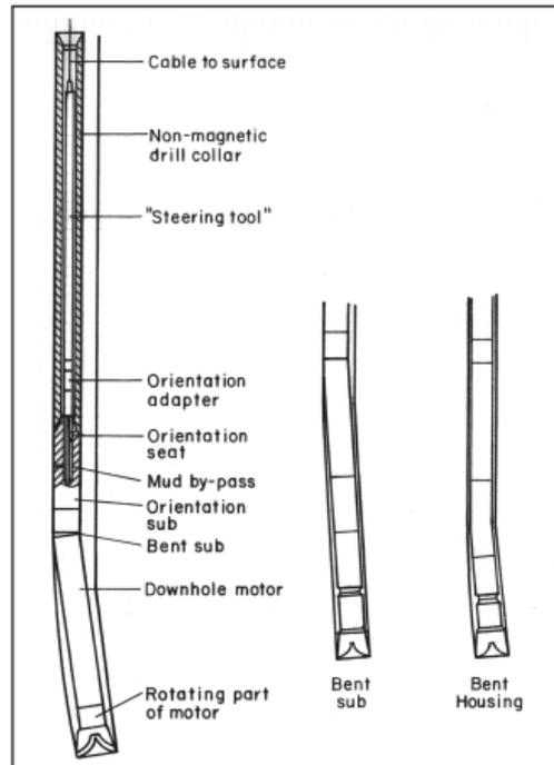
providing accurate trajectory control. Among the PDM assemblies, the most commonly used today as a deviation tool is the benthousing mud motor.
