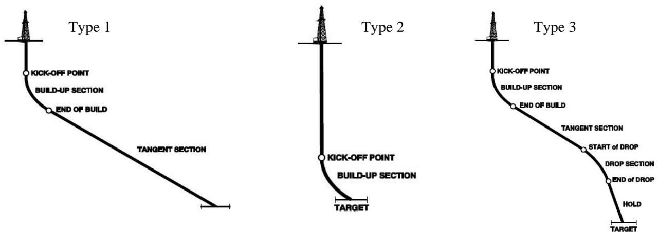
Figure 1: Types of Directional Well Profiles
