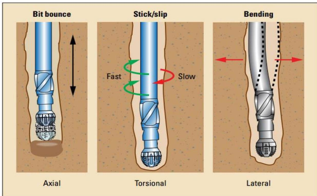
Figure11: Different categories of vibrations
