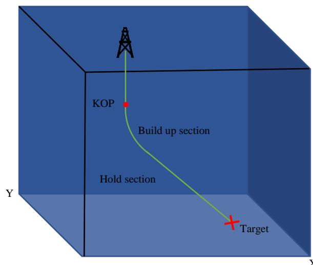
Figure 2: well trajectory design
