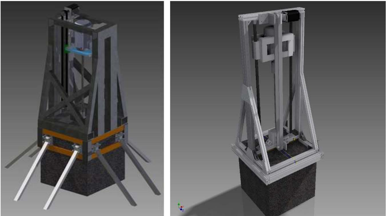
**Figure 3. CAD model of original design (left) and final design (right).**
