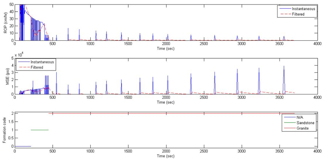
**Figure 13. ROP, MSE and formation detection for the second part of the final test where granite was encountered.**
