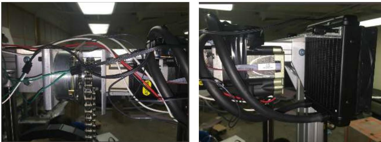
**Figure 4. Hoisting system: stepper motor, brake and chain (left); cooling unit (right).**
