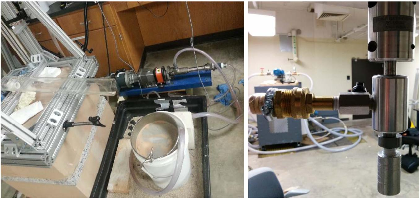
**Figure 6. Pump, mud bucket and fluid returns line (left); swivel (right).**
