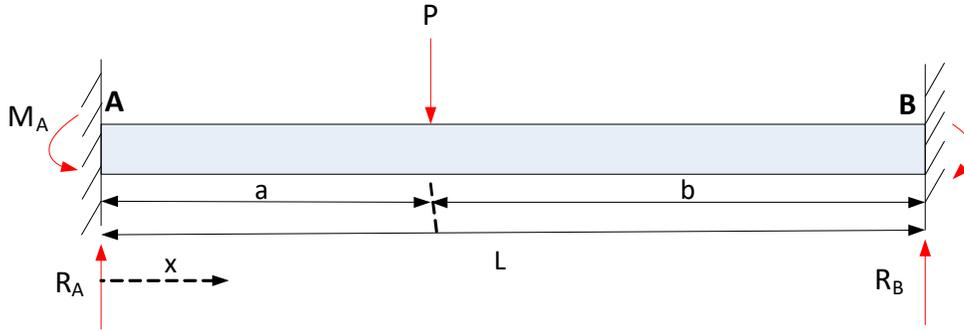
**Figure 18. Guide Rod Free Body Diagram.**
