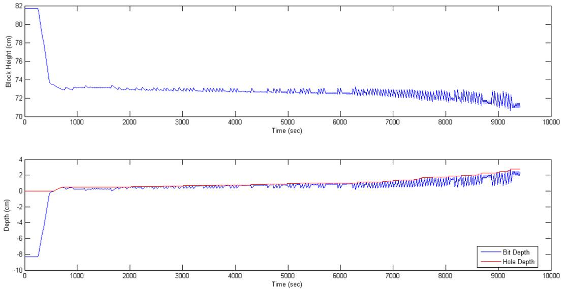
**Figure 10. Block height and bit depth for the first drilling test.**
