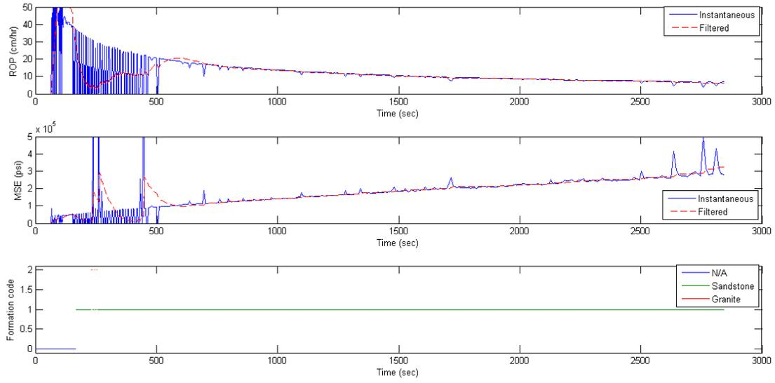
**Figure 12. ROP, MSE and formation detection for the first part of the final test through sandstone.**
