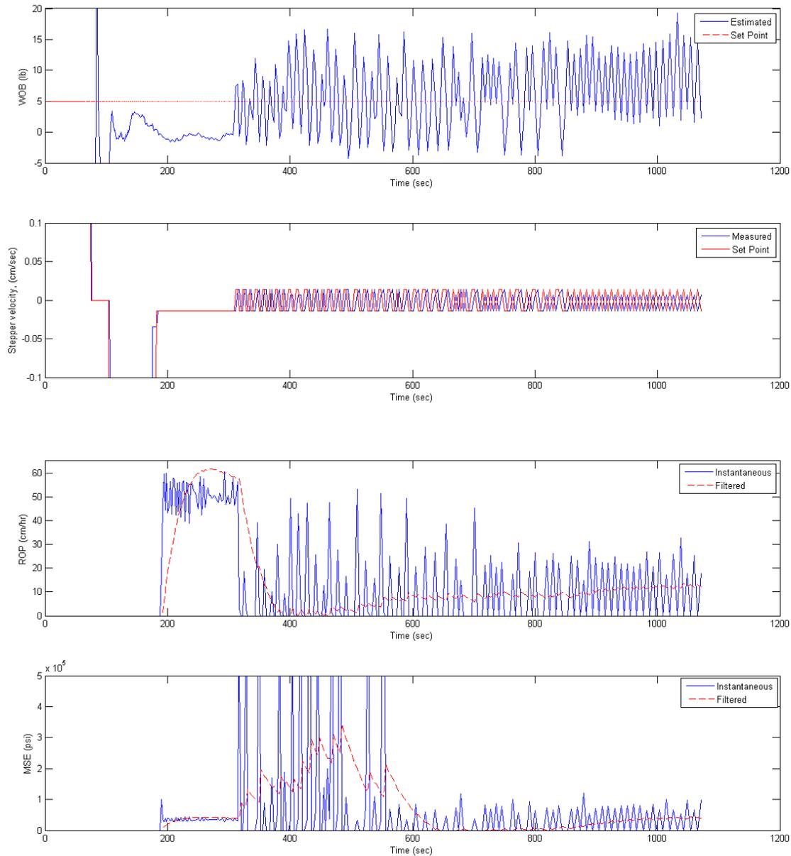
**Figure 11. WOB, draw works velocity, ROP and MSE for the second test.**
