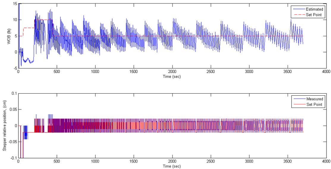
**Figure 14. WOB and draw works relative displacement for the second part of the final test.**
