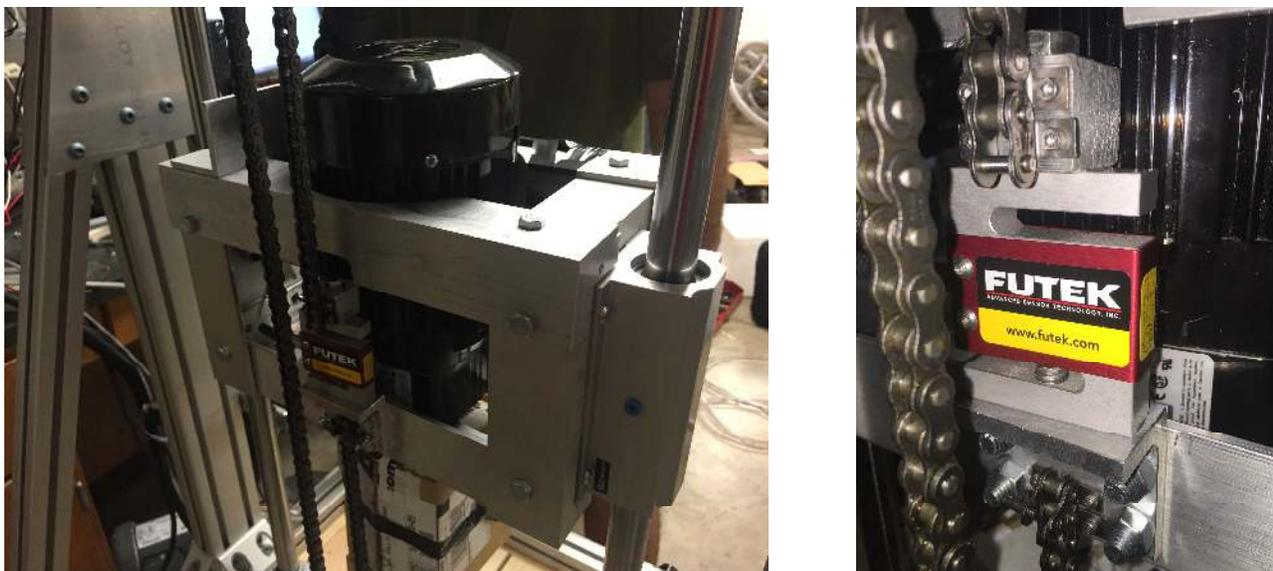
**Figure 5. Top drive carriage (left); close-up of S-beam load cell (right).**
