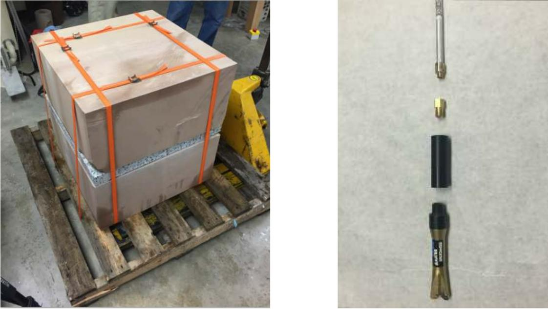
**Figure 1. Materials provided by DSATS: rock sample (left); drill string assembly (right).**
